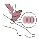
8 To make sure that you have treated all areas, release the flashes close to each other. Effective light only comes out of the light exit window. Part of the device that is in contact with your skin is slightly larger therefore there should be some overlap. However, make sure you flash the same area only once.
