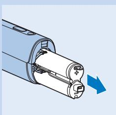
5 Shake the rechargeable batteries out of the appliance.
