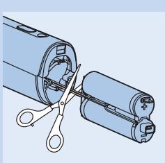
6 Cut the two wires one at a time to ensure no mishaps due to possible residual charge.
