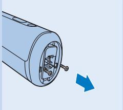
**3** Remove the bottom part of the handle and cut the two wires that connect the bottom part to the appliance.
