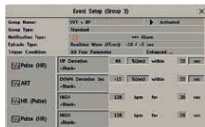
Creating event-trigger groups, using Advanced Event Surveillance, to get higher priority alerts when multi-parameter events occur.
