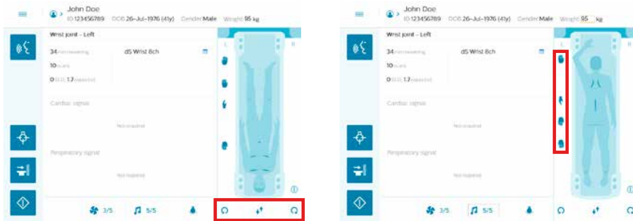
Because every patient is different, an exam strategy sometimes needs to be changed on the spot. With only one click, the position of the patient can be switched from head-first to feet-first or vice versa. In case of upper extremity studies the hand and arm positions can be adjusted just as easily.
