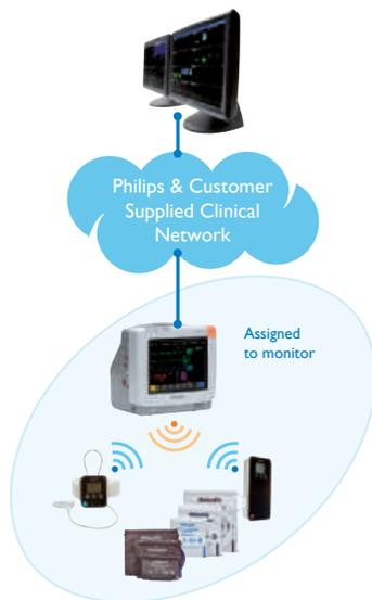
Fewer measurement cables help enhance patient mobility by eliminating the wire between the SpO<sub>2</sub>, NBP measurement device, and the monitor, while also decreasing the potential for accidental disconnect.
