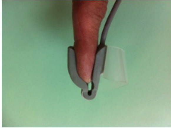
Figure 5. View of the Philips sensor showing the relatively fixed alignment of the LED and photodetector due to the components being molded into a semi-rigid silicone housing.
