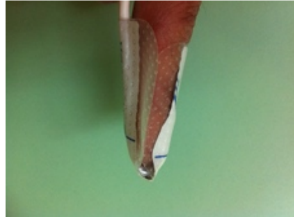
Figure 6. View of the Nellcor sensor showing misalignment of the LED and photodetector. (Represented by the blue lines, which should be directly opposing each other.)
