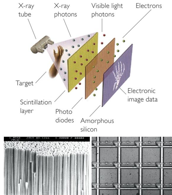
**Figure 6** Schematic depiction of the X-ray imaging process with the flat-panel detector system (top image). Close-up of the cesium-iodide (CsI) scintillator layer (lower left image) that converts the X-ray photons to optical photons. Close-up section of the amorphous silicon detector (lower right image) that converts the optical photons to electric charge that forms the electronic image data. Each detector pixel is 0.194 mm × 0.194 mm.
