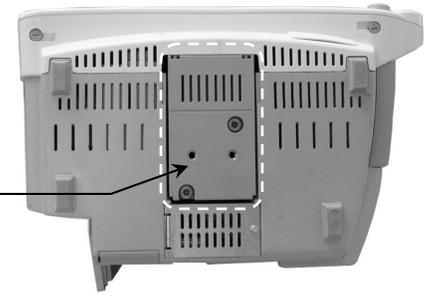
1. Fasten Philips-supplied Table Top Mount to Mounting Adapter with one (1) M6 x 12mm FHMS and two (2) M6 x 8mm FHMS (see below).
