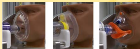
Figure 3. Photos of each VHC-facemask system tested under 0° deg face replica tilt, 1.9 kg applied force for 1 simulated pediatric breath: (Left) OptiChamber Diamond-LiteTouch, (Middle) AeroChamber Z Stat-ComfortSeal, (Right) Vortex-Spinner Duck.
