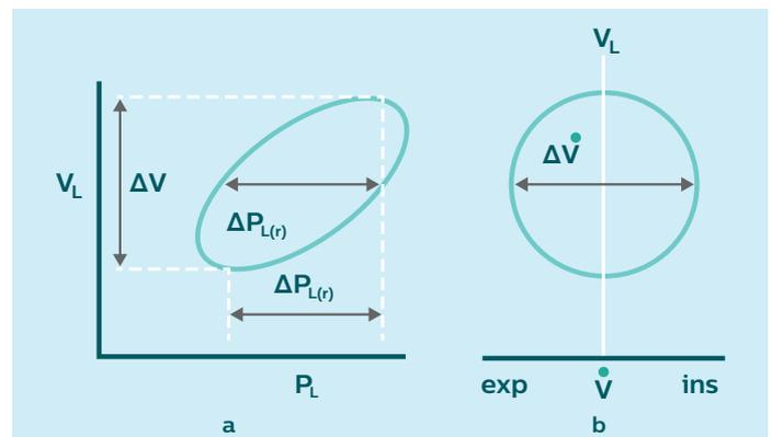
**Figure 2** (a) Pressure volume and (b) flow-volume curves for the lung in a single breath volume excursion ( $\Delta V$ ) and elastic pressure change ( $\Delta P_{L(e)}$ ) are used to compute compliance, and the inspiratory-expiratory flow difference ( $\Delta \dot{V}$ ) and resistive pressure difference ( $\Delta P_{L(r)}$ ) are used to compute resistance (adapted from Loring, 1998).
